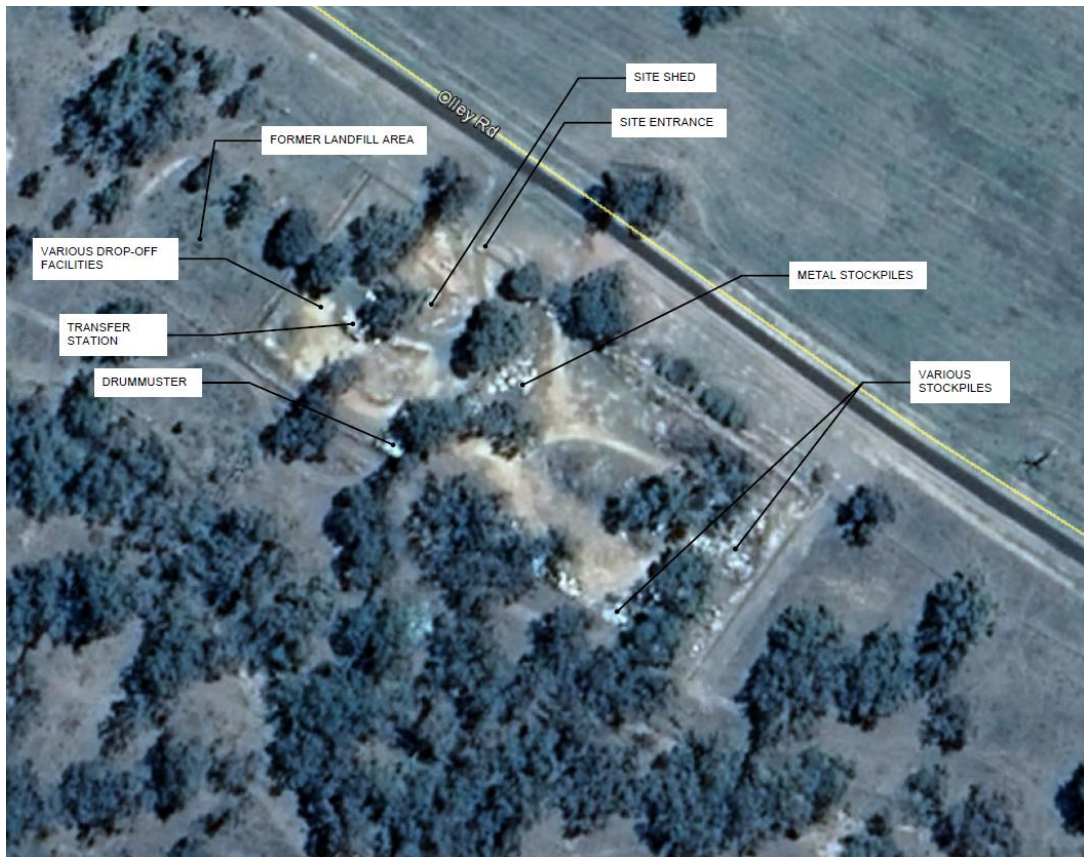
Figure 4.3 Tomingley Transfer Station existing site layout
